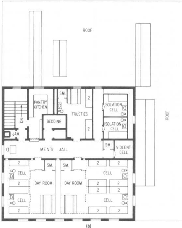
Fig. 3 (cont.) Plan of police station for city of 15,000 population. Building 6,000 sq ft. (a) First floor plan. (b) Second floor plan.
