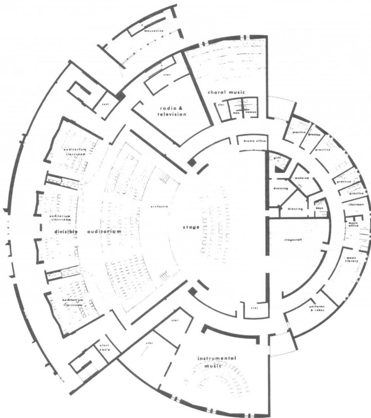
Fig. 6 Divisible auditoriums provide a means of increasing the use of large areas. Huron High School, Ann Arbor, Mich. Lane, Riebe, Weiland, Architects.
