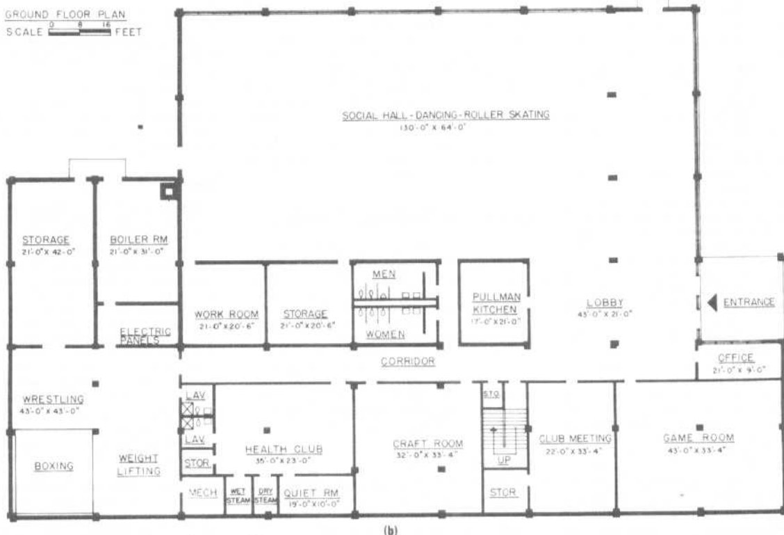
Fig. 1 (cont.) Collett Street Recreation Center, Morganton, N.C.
