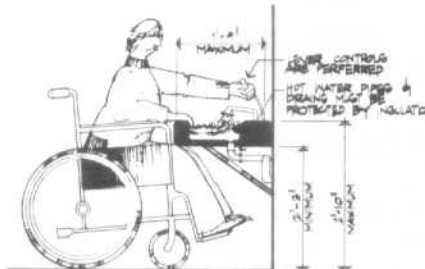
Fig. 12 Sink with knee space. Source: "Handbook for Design: Specially Adapted Housing," VA Pamphlet 26-13, Veterans Administration, Washington, D.C., 1978.
