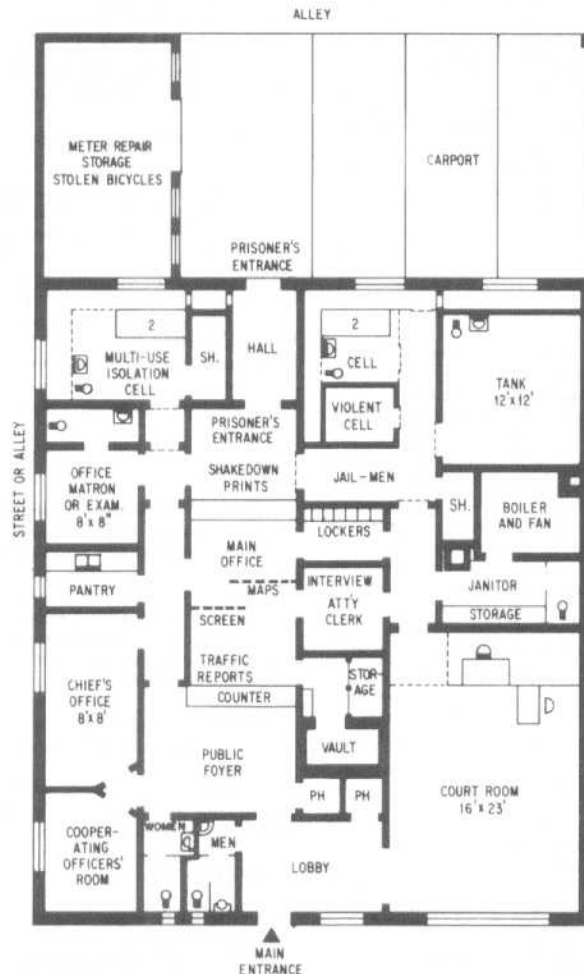
Fig. 1 Plan of police station for city of 3,500 population. One story, lot 48 by 74 ft, building 2,784 sq ft.
