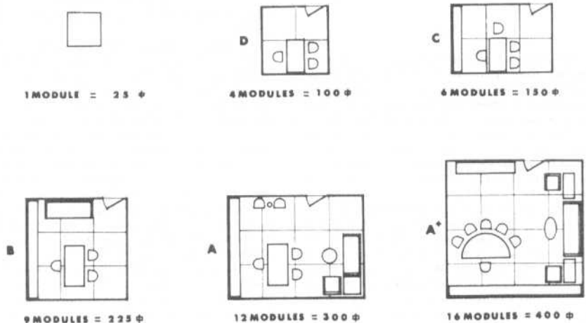
Fig. 1 Typical modular office plans.
