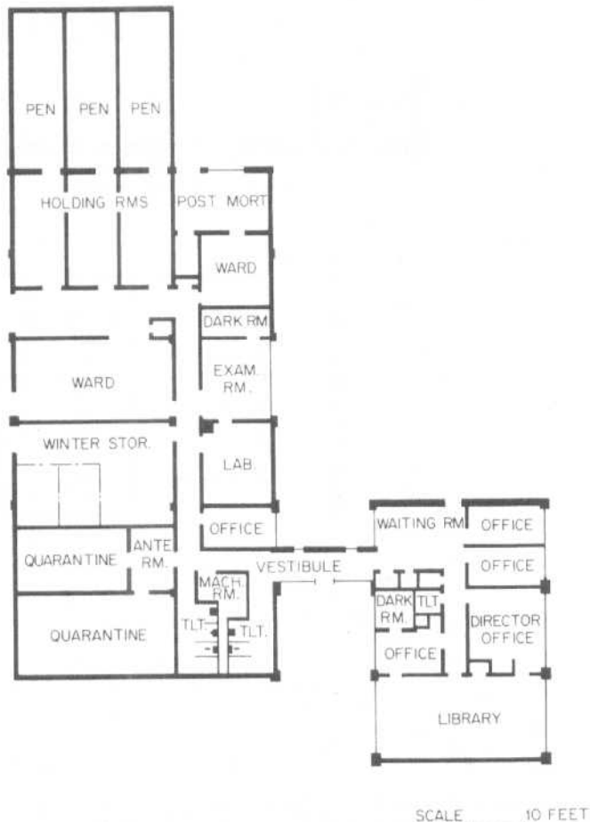
Fig. 7 A combination administration and hospital building. Facilities include a library, offices, quarantine and ward rooms, laboratory, pharmacy, and winter quarters. Zoo buildings, especially service facilities, require a careful selection of construction materials, particularly those which will stand up under constant humidity and abrasion of daily cleaning. (Franklin Park Zoo, Boston.)
