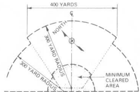
SHOTFALL DANGER ZONE
